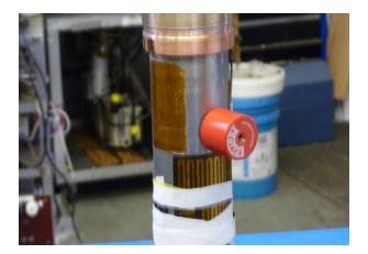
The Cryostat was assembled and tested with muons in May 2015. The test was performed with the Lampf spectrometer with the cryostat installed axially on the M20D beam line (runs 25008 through 25024)
