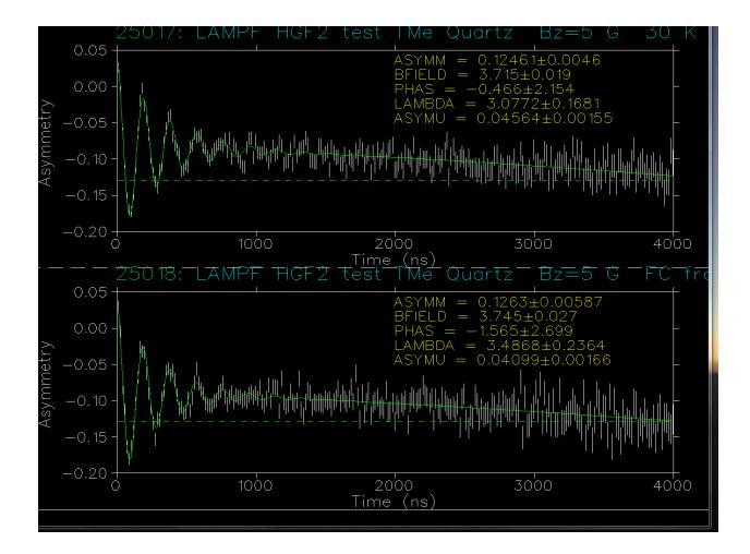
Next the quartz sample was zero field cooled from 30 K to 3 K, a magnetic field Bz=5.1 G was applied and the frequency of muonium measured at 3 K. This was followed by warming the sample back to 30 K and comparing the value of the fields (5.11 G @ 3 K and 5.17 G @ 30 K). It is clear that no magnetic shielding is present.
