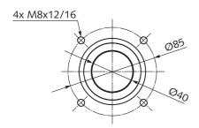
In the case of long discharge lines, the line cross-section should be larger than the exhaust flange in order to prevent a drop in the performance of the vacuum pump. If you have any doubts, contact your Busch representative.
