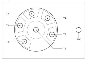
Star motor connection (High voltage) 400V:
