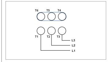
Delta motor connection (Low voltage) 200V:
