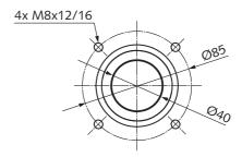
In case of long inlet lines the pipe diameter should be larger than the inlet flange to prevent a drop in the performance of the vacuum pump. If you have any doubts, contact your Busch representative.
